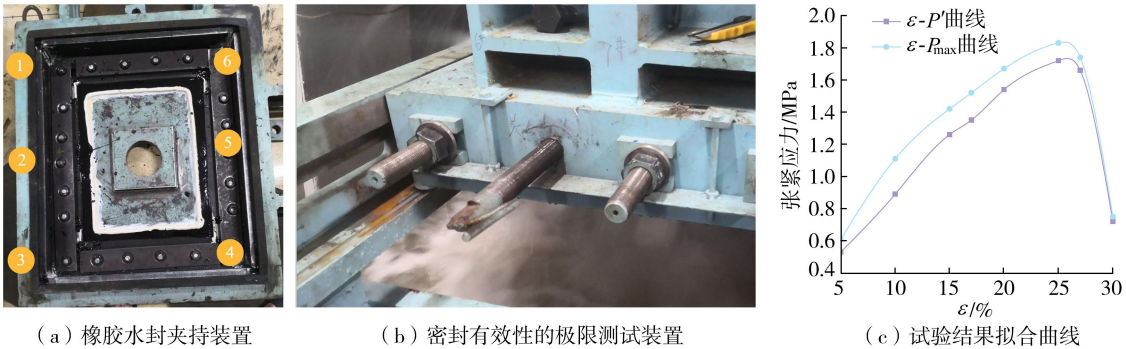
图6 水封密封有效性验证试验 Fig.6 Verification test for sealing effectiveness of water seal
