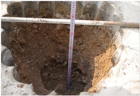
图8 碎石垫层厚度较大及松散块石充填
