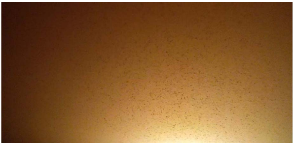
图1 沉降筒微距拍摄泥沙絮凝现象 Fig.1 Microscale photography of sediment flocculation phenomenon in settling tube
