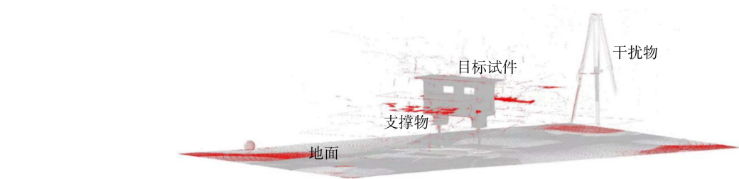
图 4 初始点云与降噪后点云对比 Fig. 4 Comparison of initial point clouds and denoised point clouds
