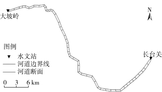
图 3 淮河大坡岭—长台关段河道概化 Fig.3 Schematic diagram of Dapoling-Changtaiguan section along Huaihe River
