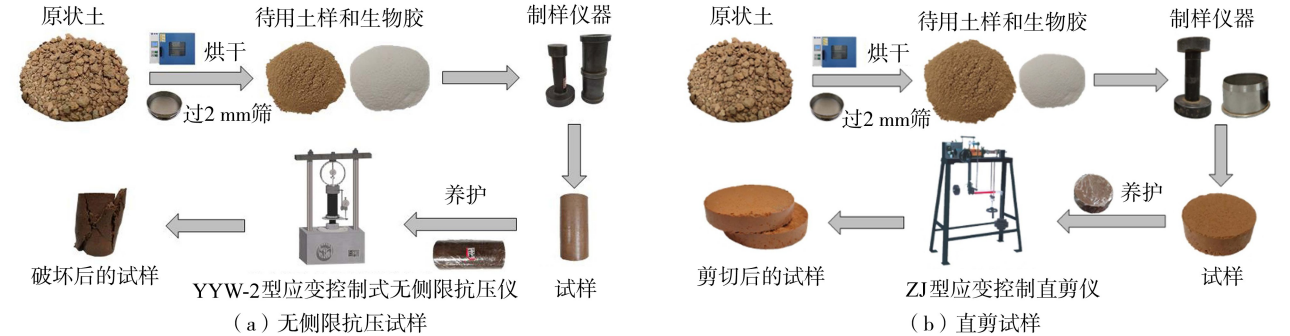
图 4 试样制备过程 Fig.4 Sample preparation process
