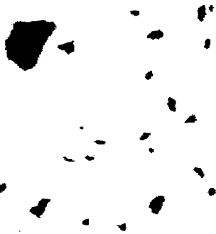
图 3 拉断骨料分布 Fig.3 Distribution of fractured aggregate
