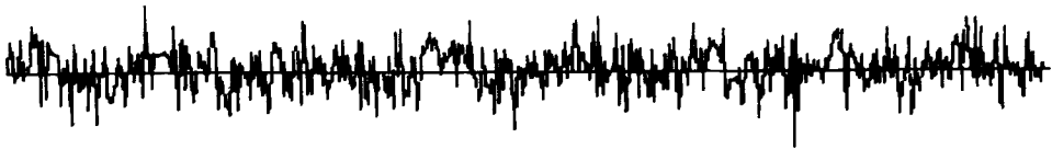
图 3 正弦函数叠加 Gauss 分布随机数 Fig.3 The combined series of a sine-function component and an independent stochastic component
