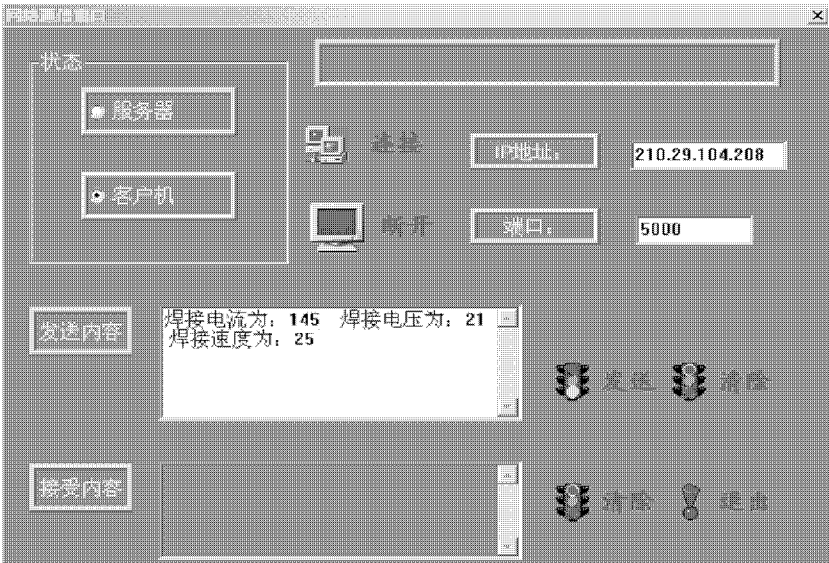
图 3 专家系统与机器人通信的操作界面 Fig.3 Interface of communication between expert system and robot
