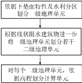
图1 洪涝特性区划流程 Fig.1 Flow chart for flood and waterlogging behavior regionalization
