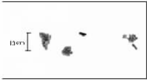
图6 活性炭滤柱出水中炭粒照片(放大400倍) Fig.6 Picture of carbon particles in effluent from activated carbon filtration(400 times enlarged)
