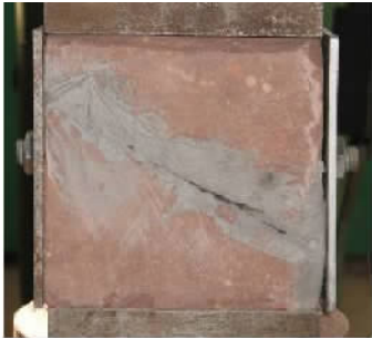
图 2 加工的裂隙砂岩试样 Fig. 2 Sandstone sample with single crack
