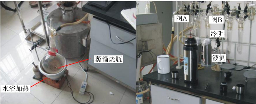
图 3 真空蒸馏法提取土壤水装置 Fig. 3 Soil water extracting device using vacuum method
