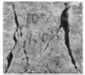
图 15 混凝土压缩破坏形态 Fig. 15 The failure mode under uniaxial compression for concrete sample
