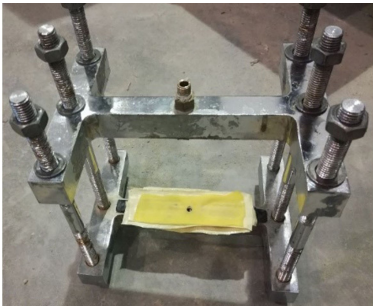
图2 高压水密封装置 Fig.2 High water pressure sealing device
