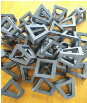
图 1 四棱台透水框架构件 Fig.1 Water permeable frame member of tetrahedron permeable frame
