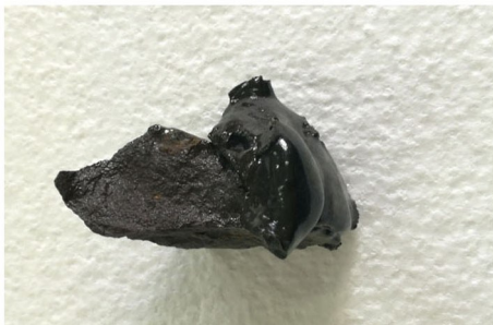
图 3 1200 °C煅烧水淬后火山岩玻璃质化照片 Fig.3 Vitrification photo of volcanic rock after 1200 °C calcination and water quench
