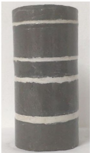
图1 含软弱夹层的层状岩体试样 Fig.1 Layered rock mass samples with soft interlayers
