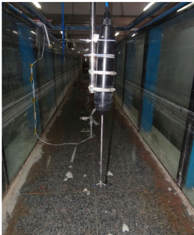
(a) ADV现场安装
